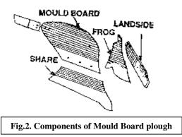
i) General purpose - It is a mouldboard having medium curvature lying between stubble and sod. The sloping of the surface is gradual. It turns the well defined furrow slice and pulverises the soil thoroughly. It has a fairly long mouldboard with a gradual twist, the surface being slightly convex.
