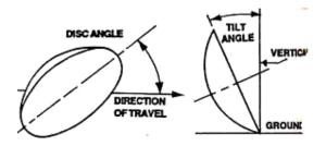
Fig.6. Angles of disc plough
