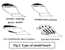
iv) Slat type - It is a mouldboard whose surface is made of slats placed along the length of the mouldboard, so that there are gaps between the slats. This type of mouldboard is often used, where the soil is sticky, because the solid mouldboard does not scour well in sticky soils.
